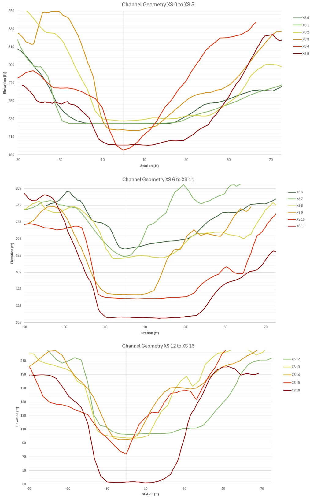
Figure 4-29. Vodopad River cross-sectional profiles (thalweg at station 0)
